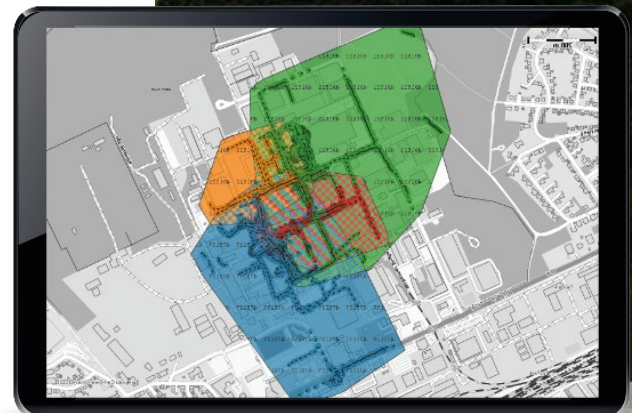
Private 5G networks: visualization of radio cells, expansion and overlap
